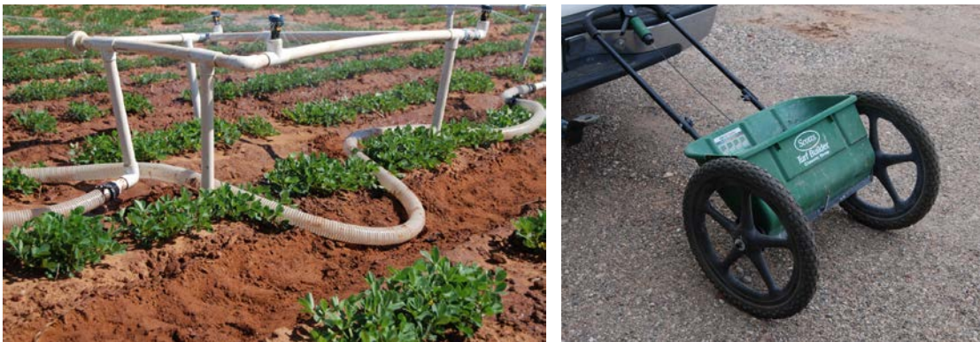
Figure 6. Chemigation simulator (left) and modified drop spreader (right) used to administer liquid calcium and gypsum treatments, respectively in field studies.
